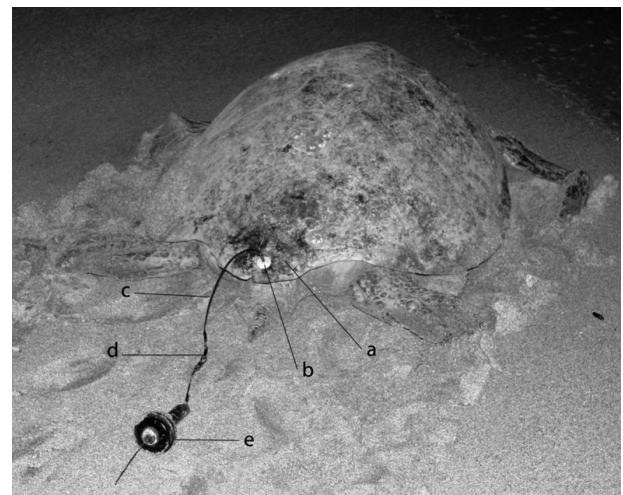
Figure 2 Satellite transmitter attachment to an East Pacific green turtle ( Chelonia mydas ): (a) posterior marginal scute; (b) upper plastic button; (c) flexible lanyard (400 lb monofilament fishing line); (d) Corrosive link with metallic crimps and swivel; and (e) satellite transmitter (Mk 10 PAT tag, programmed for opportunistic transmissions).
